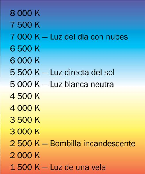
A vertical color gradient bar on the right side of the page, transitioning from dark blue at the top to orange at the bottom. It serves as a visual scale for color temperatures in Kelvin (K).
