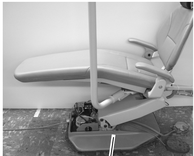
Dental Light Cable from the Lift Arm to the Floor Box or Pump Housing
