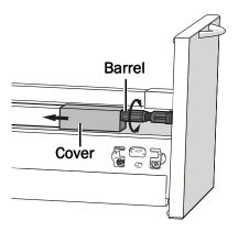
**4** Front to Back Tilt (Gallery Rails only) - Slide the covers and rotate the barrels.
