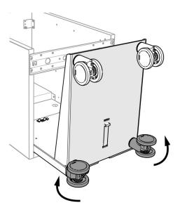
**3** Rotate the back wheels so that the base lays flat against the cart.
