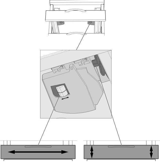
**1 Side to Side:** Rotate all barrels in the direction you want the drawer face to move.
