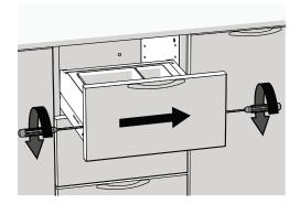
**3 Side to Side:** On both sides, adjust the screws closest to the face of the drawer. Make sure to move both screws in equal increments. The direction shown moves the drawer face to the right.
